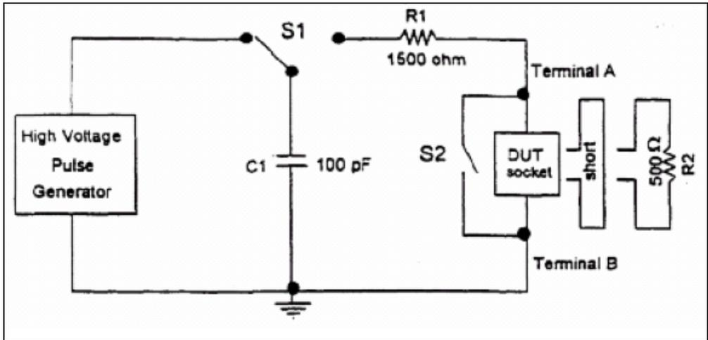
Figure 1: Typical equivalent HBM ESD circuit
