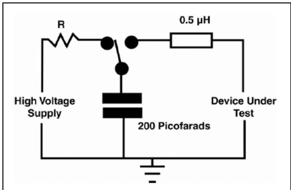
Figure 2: Typical Machine Model circuit diagram
