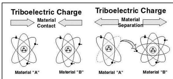
Figure 1: Principle of Triboelectric charge
